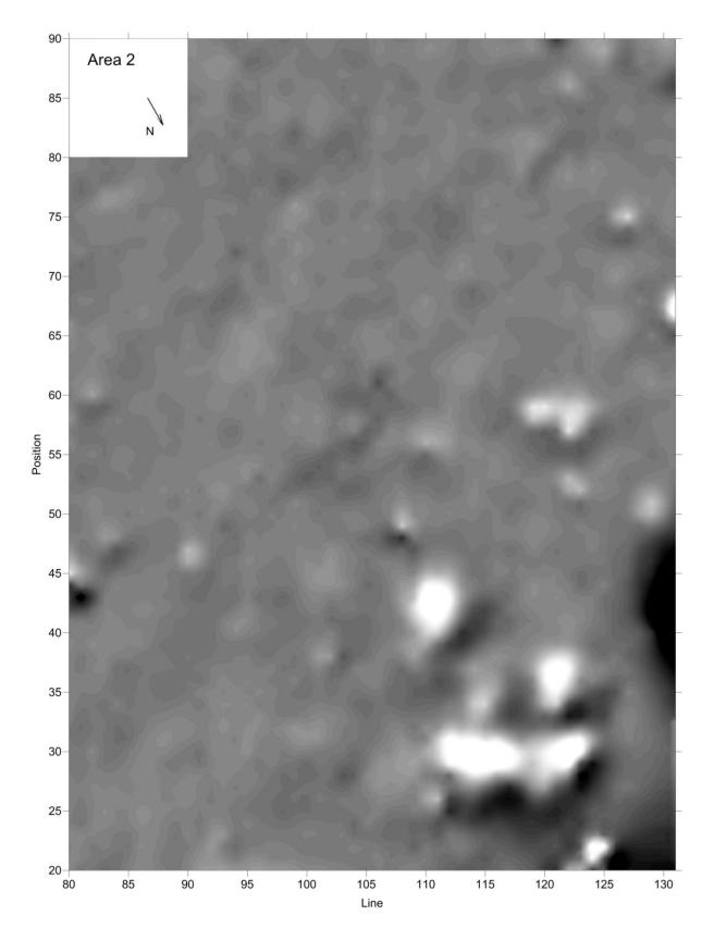
The anomaly near (130, 40) is caused by metal parts of a bench and a nearby railing. The upper left part of the area does not show significant anomalies, it is mostly bedrock very near the surface or at the surface. An experienced interpreter knowing the site might evaluate significance of the diagonal trend of isolines.
