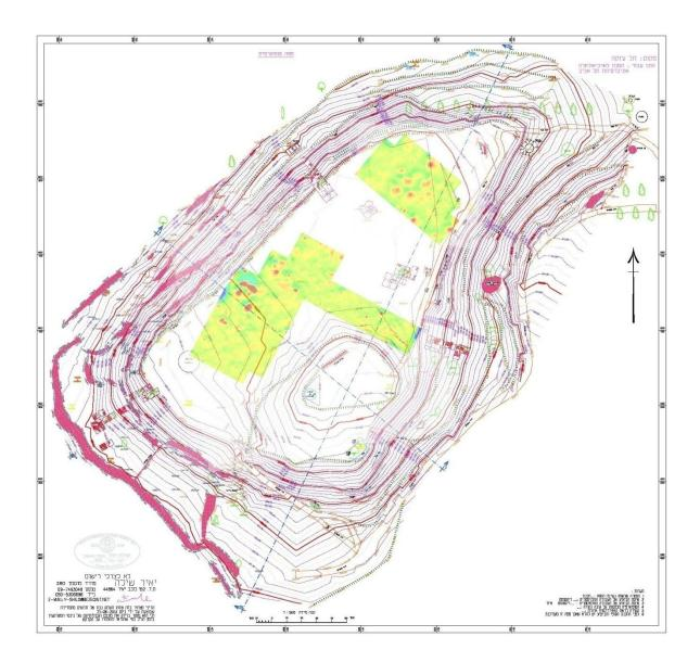
Anomalies of the gradient of the magnetic field in measured areas 1-4
