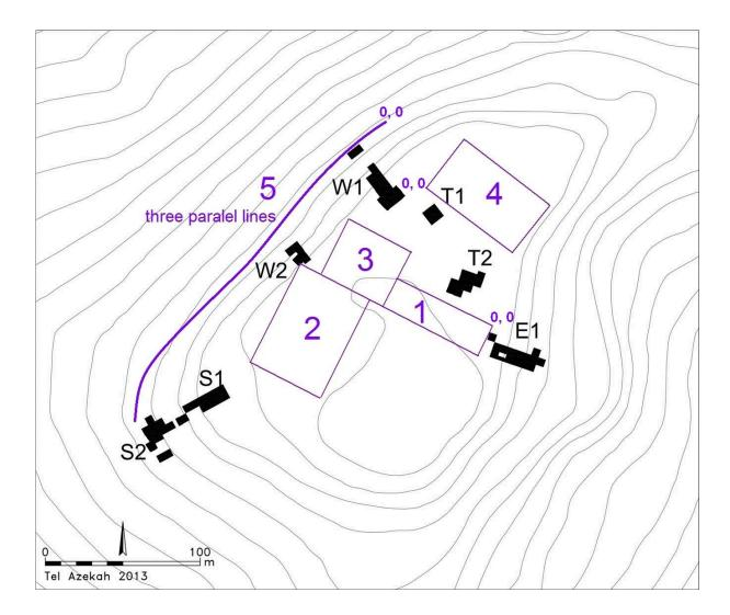
Measured areas 1 to 4 are located at the terrace. Area 5 is three parallel lines 1 m apart. They follow an old path climbing slowly from the bottom of S2 to the bottom of W1 and behind.
